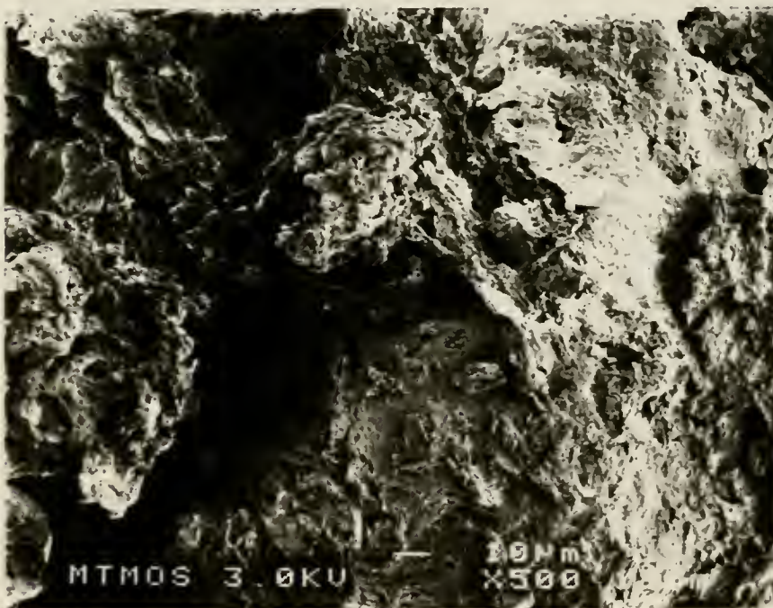
Figure 2.9 SEM photomicrograph of facsimile treated with methyl trimethoxysilane monomer (MTMOS) and etched with 1M HCl. 3.0KV, 500X magnification.
